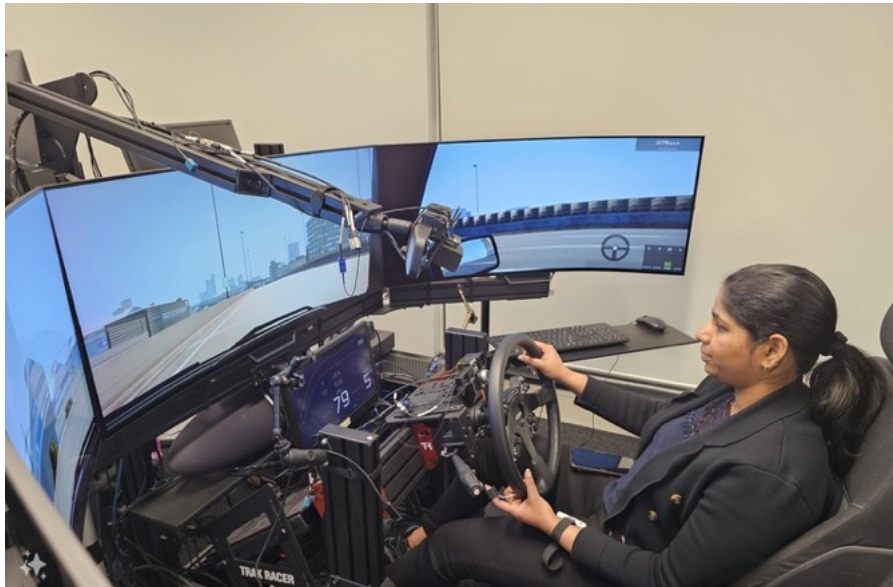
Figure 16: The Seeing Machines indoor data collection simulator used for the data collection campaign. Subjects physiological signals are recorded through the use of ECG electrodes and a finger clip PPG sensor. The physiological sensing data is synchronised with three camera streams: two located on the IC and one located in the RVM position.
