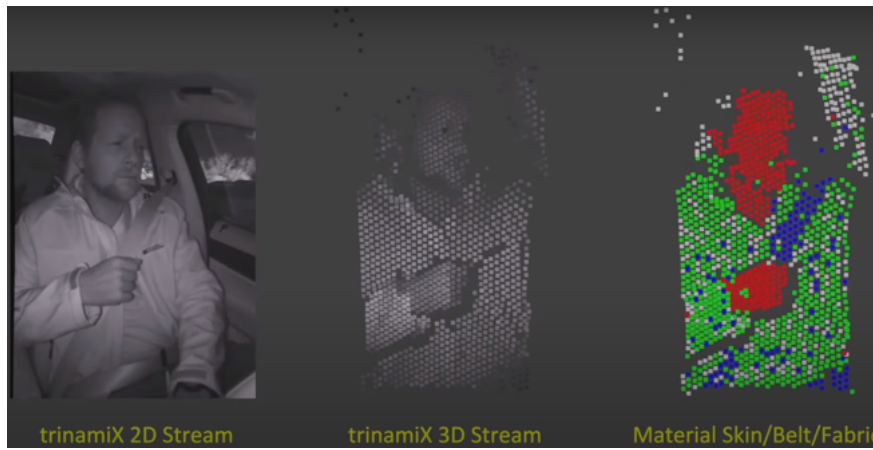
Figure 11: An example of trinamiX GmbH beam profile analysis material classification technique deployed in a DMS application scenario [14].
