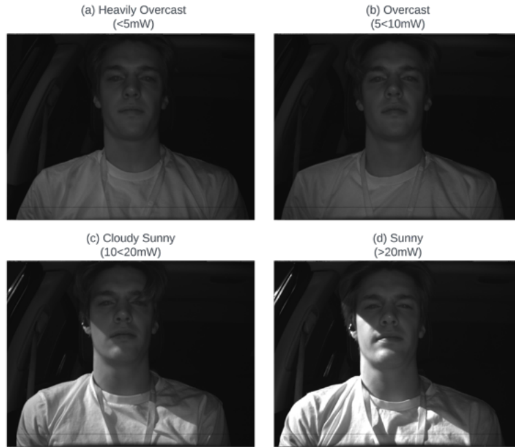
Figure 53: Ambient light categories used for categorising of the ambient light evaluation datasets. For each category, an example of a corresponding image is provided.
