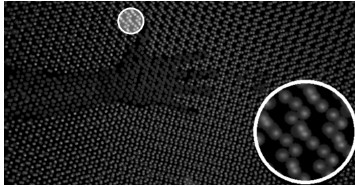
Figure 21: Masked dots image. Virtually all image content is zeroed excluding the beam profile of each dot.
