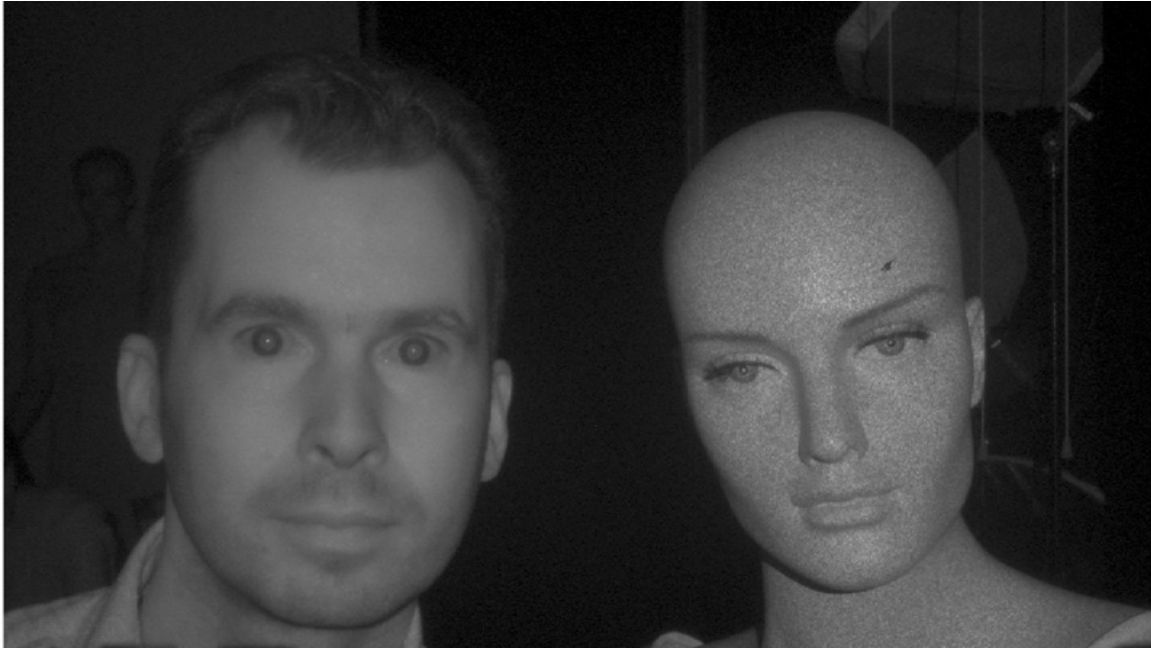
Figure 2: Coherent light interference as appears on translucent organic skin (left) versus an opaque plastic dummy (right). Notice that the interference operations are much more prevalent on the opaque surface while they are mitigated on the translucent skin.
